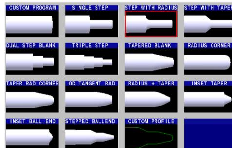
The Model 2150™ has the ability to dress grinding wheels in cycle with automatic size compensation for wheel wear after dress. Whether dressing a simple flat wheel or an intricate profile, dressing can be automatically executed during grind cycles as controlled by the machine's operator.
