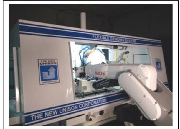
The Model 2150™ utilizes Unison's proprietary software and control which allows your operator to customize centerless grinding, such as through feed, infeed & secondary operations, including plunge grinding, tapers and profile grinding of cylindrical parts with a range of diameters from 0.005" (.127mm) to 5" (127mm).
